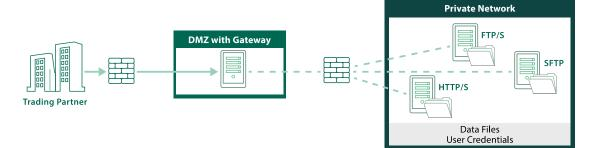
For example, a company may require that any FTP/S or SFTP file transfer requests from within the private network must pass through the gateway's forward proxy. The firewall rules could be configured to allow only the gateway's address (IP and port) for FTP/S or SFTP traffic, blocking all other addresses from performing those requests.
