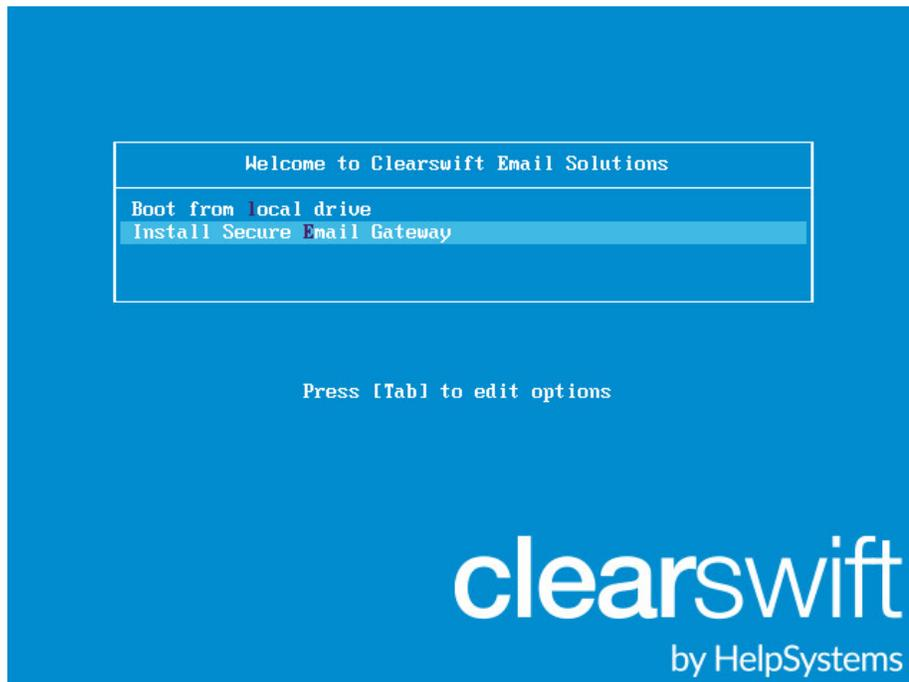
2. Use the arrow keys or keyboard shortcuts to select **Install Secure Email Gateway** from the menu. Press the **Enter** key to select the installation. The install process begins and starts the Red Hat Installation Wizard.
